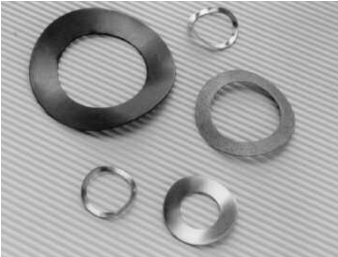
Fig. 1. Cylindrically Curved Spring washers are used where flexibility is important and loads are light. Maximum height should be less than one-half of the outside diameter.
