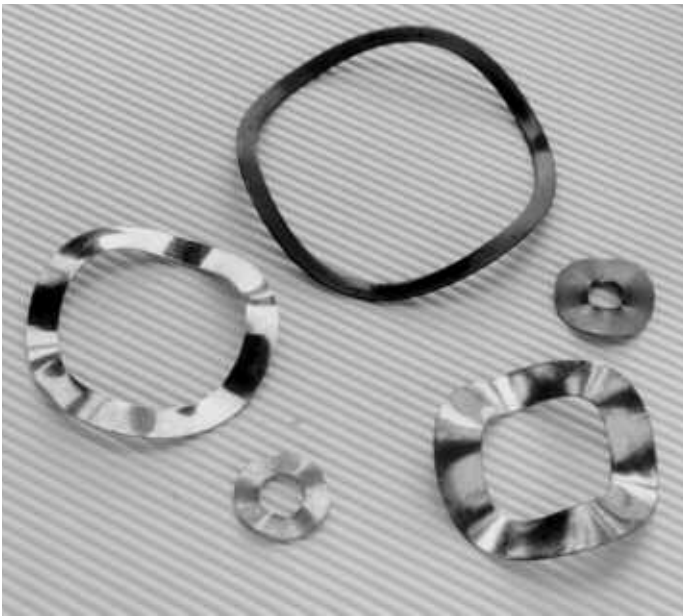
Fig. 4. Wave spring washers are effective when the load is static or the working range deflection is small, and the allowable axial space for installation is limited.
